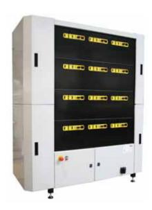
The SBT8050 is a 12-Channel Battery Tester, ideal for testing and evaluating HEV as well as industrial battery modules and packs. Our equipment is designed for both laboratory and production scale applications, including formation and ranking.
